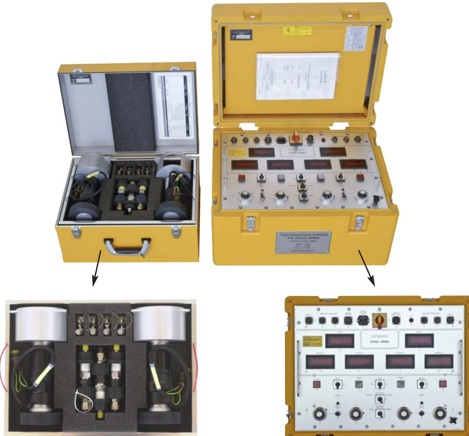
The equipment is designed to test on aircraft the anti-skid systems of the following aircraft types A320, AMX, C-27J, EF-2000 and G-222.
