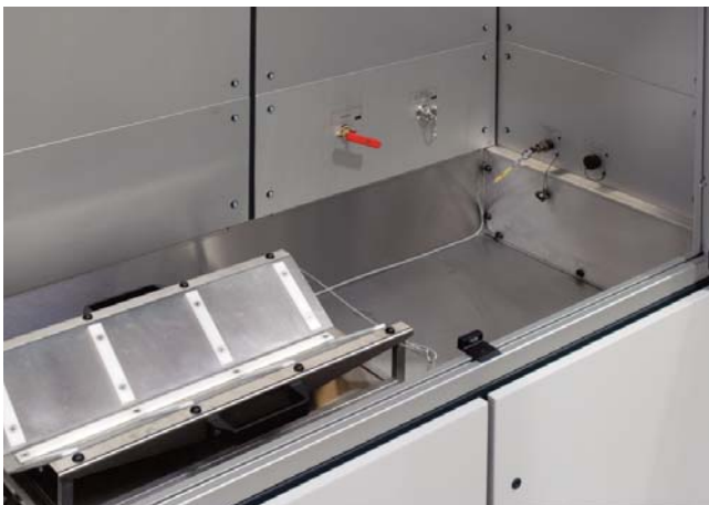
Filling room with weighing platforms and stainless steel adaptations
