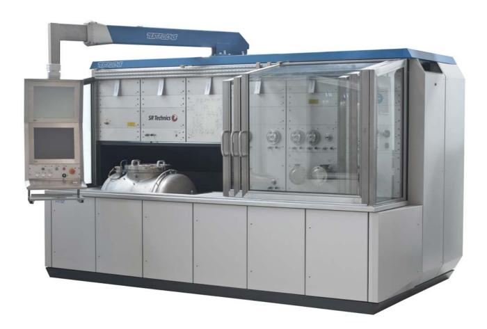
The test stand is developed to test fuel-supply pumps (e.g. fuel booster pumps) and heat exchangers in accordance with ATA Chapter 28
