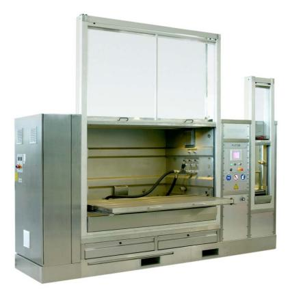
To test aircraft components, e.g. oil nozzle, bearing dampers of engine bearings.
