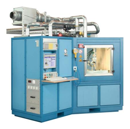
Designed to test and adjust the characteristic parameters of fuel nozzles like flow stability, flow rates, spray angle, diffusion and leakage.
