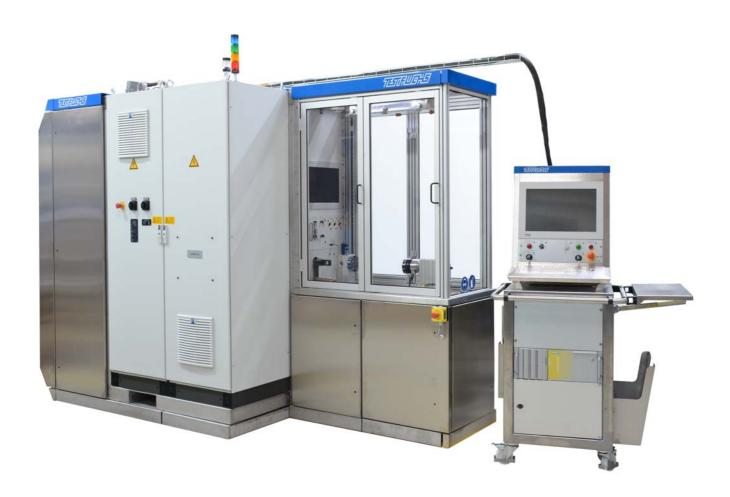
The test stand is developed for fully automatic testing of Hydraulic Flight Control Units (HFCUs) of the AIRBUS A320 in accordance with ATA Chapter 27.
