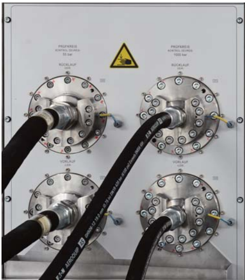
Hydraulically operated quick release latches
