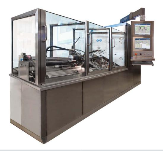
This test bench is developed to test the function of flight control units for 3000 and 5000psi systems for aircraft types like:
