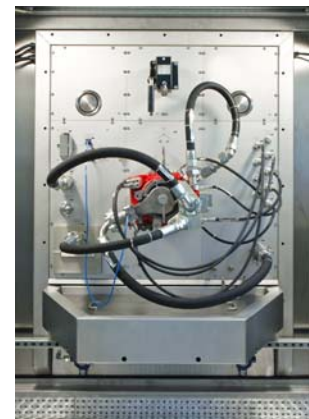
UUT on the pump test stand
