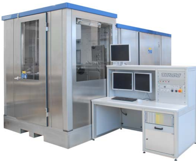
Pump Test Station
