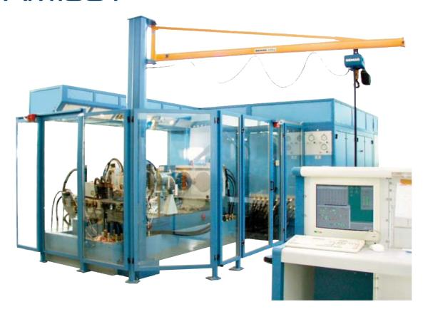
This combined test system provides for testing of Aircraft Mounted Accessory Drives, Generator Converter Units, Transmission Units, generators, and regulators. It serves to check identification data, such as pressure, flow, temperature, torque, force, speed, angle of rotation, vibration, voltage, current, frequency, and power.
