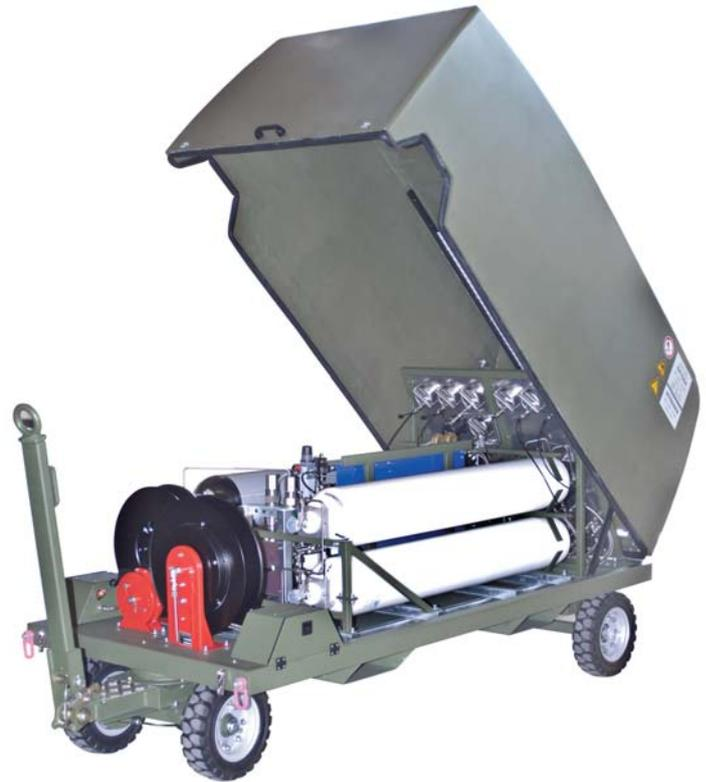
Regulable oxygen supply for the aircraft
