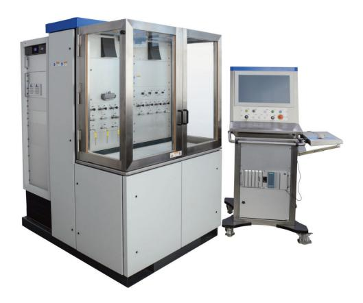
The system serves to check pilot valves using the media MIL H-5606H and MIL-83282.
