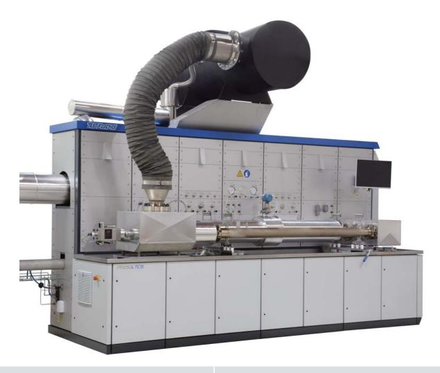
The test stand is developed for universal testing of High-Flow Components (e.g. valves) and their parameters (pressure, temperature, flow and leakage) in accordance with ATA Chapter 36.
