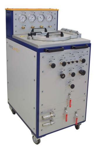
Developed for testing actuators in a dip tank filled with water.
