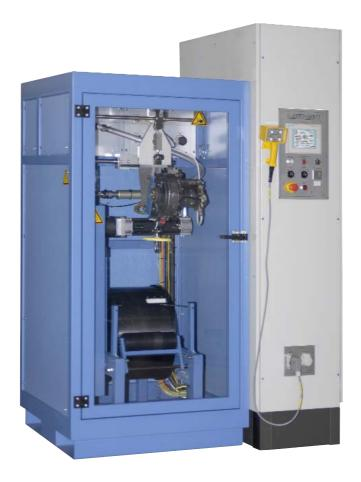
The test bench is developed for testing the ALOUETTE III Rescue Winch.
