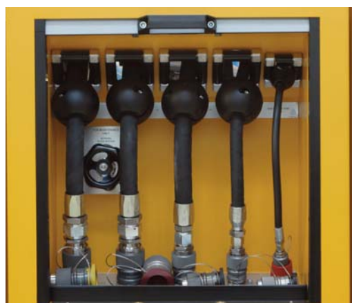
Colour coded test connections
