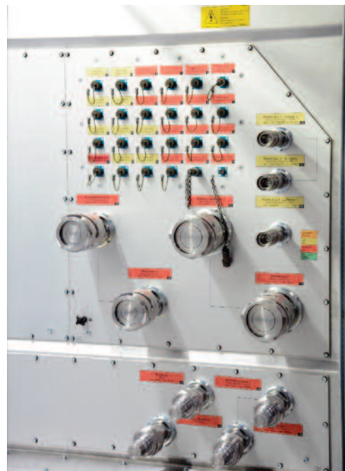
Anodized front plate with colour coded UUT connections (depending on operating medium)
