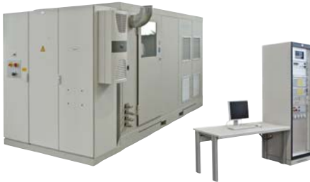
>TE-FLSA1< (part of >EHPSAT6-8<) High Pressure Test, Flushing and Particle Measuring
