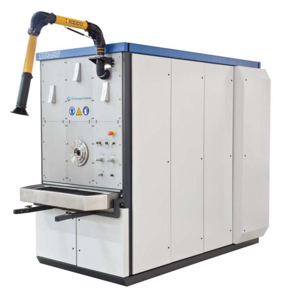
The test stand is developed for testing the characteristics of Air Turbine Starters, such as e.g.: pressure, flow, temperature, rotational speed and torque.
