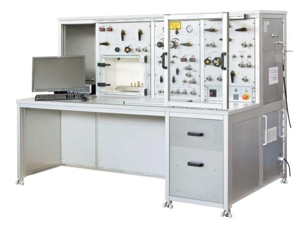
This test stand is developed to test oxygen components and regulators of all current aircraft and characteristics e.g. proof pressure, flow and leak rate.
