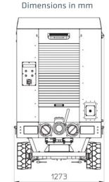
\* Variant trailer platform: approx. 4800x1500x2200mm (LxWxH) \* Variant van: approx. 3043x1273x1690mm (LxWxH)
