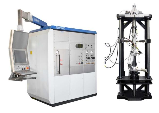
The test stand is developed for filling, regulating and testing of vibration dampers and hydraulic cylinders of the A/C Eurofighter and Tornado.
