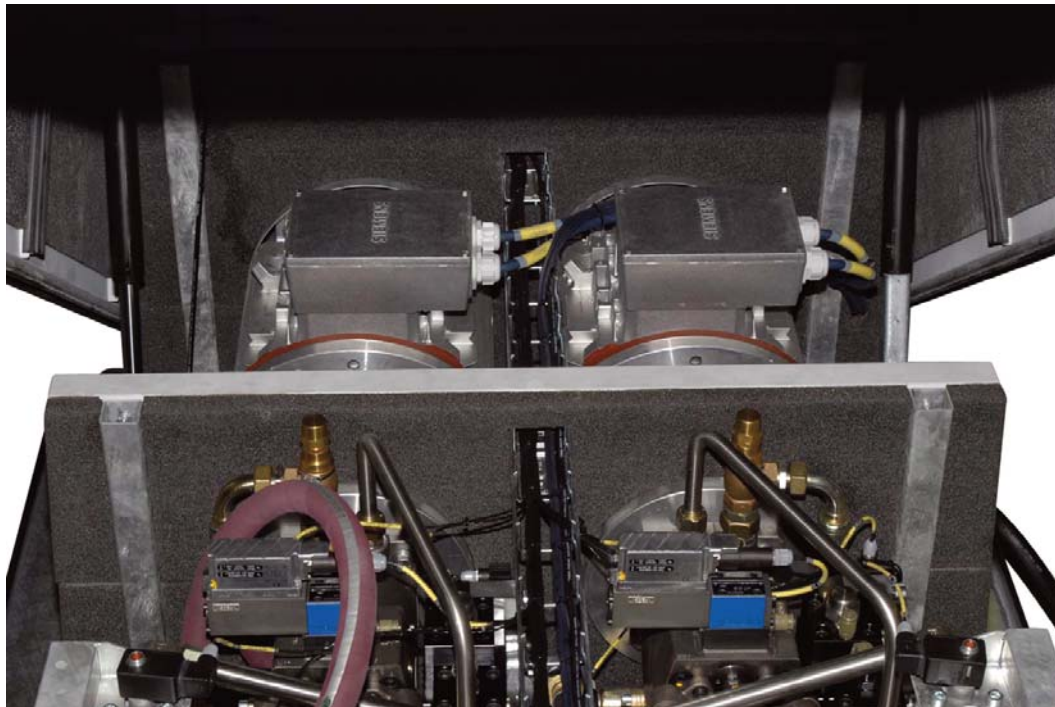
Figure shows interior view of an >HGPU< with dual system. The two electric pump drive motors for the two independent hydraulic circuits drive the DUAL SYSTEM without interconnection with each other.
