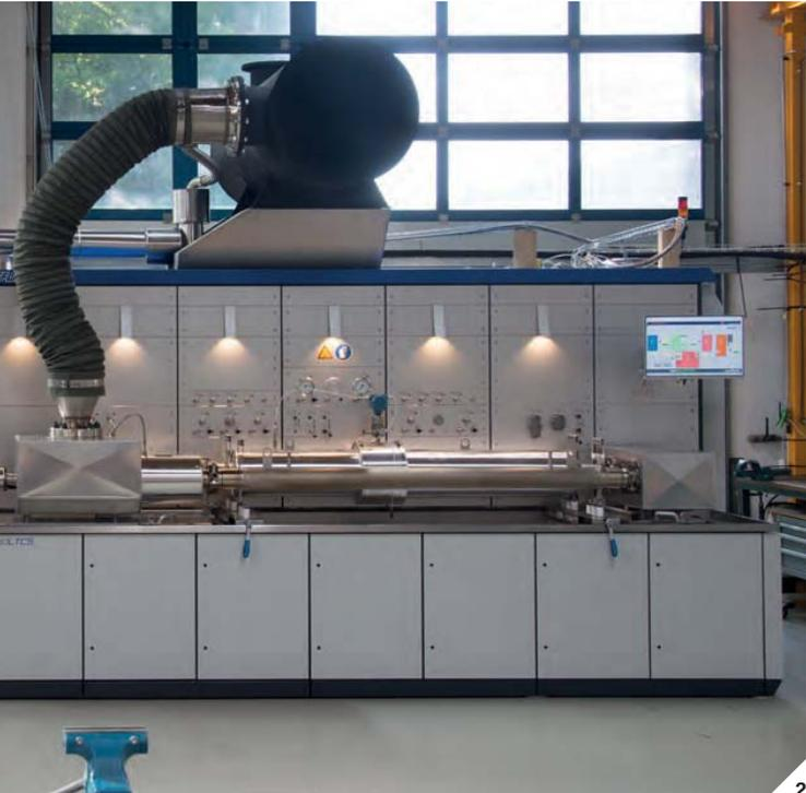
system and the precise accuracy of the parameters are greatly improved by the in-house designed valves. These operate with positioners and replaceable valve disks and feature excellent position feedback, <40ms valve actuation, 1/10,000th positioning accuracy over the operational range (a 20mm operating displacement would result in an accuracy of 2µm) and an integrated superimposed feedback control loop.
